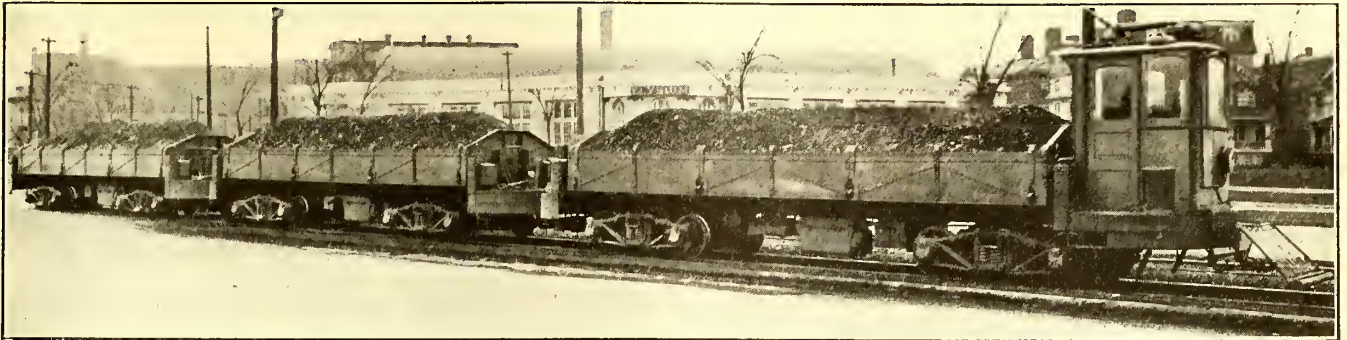
This All Steel Train of Differential Electric Dumping Cars belongs to the Cleveland Railway Co., Cleveland, Ohio. They save enough labor within one year to pay for themselves. They make more money than passenger cars.
